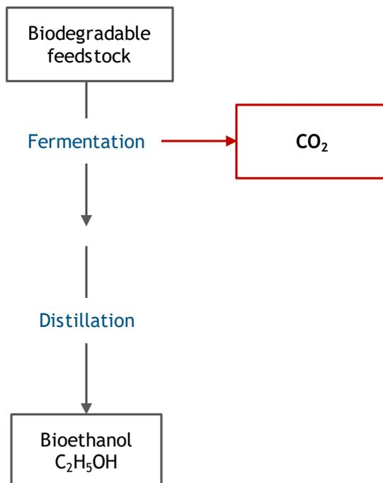
Figure 2: Bioethanol production (process simplified) heated with water and specific enzymes which bring out the natural sugars in the 'mash'.
